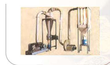
These pin mills have both discs rotating either in one direction or opposite direction. The relative speed is very critical and is maintained within design limits. The discs are rotated by two independent motors, by two independent motors. These pin mills are without These pin mills are without screen and produce fine particle size
